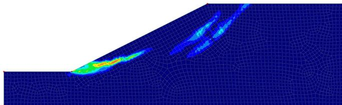
**Figure 3: Effective shear strain with scaled strength parameters (FS = 0.96)**
