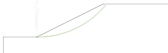
**Figure 4: Failure surface using Bishop Method (FS = 0.94)**
