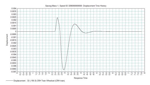
The graph shows that the sprung mass representing the body of the last wheelset of the train displaces almost 6.7 mm from its static position while it is over the continuous beam before the damping of the spring-mass system quickly damps out the body motion after the wheelset leaves the structure.
